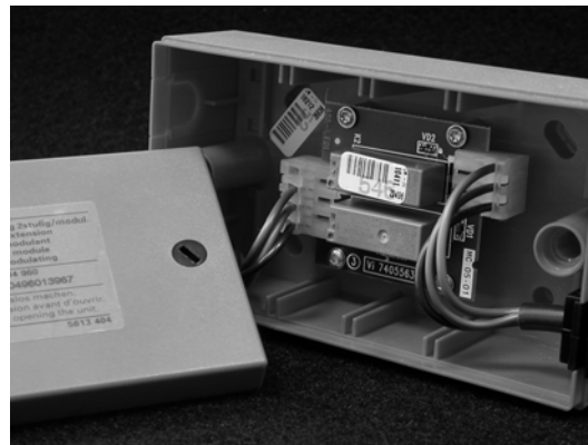
Below: Inside of 2 stage/modulating control showing relays
