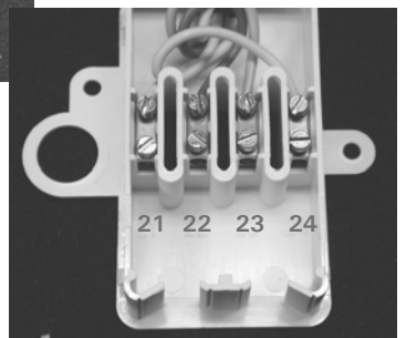
Terminals shown inside of RIKO. Note 21 to 24 from left to right.
