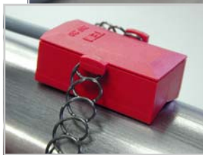
Picture above and to left show strap-on sensor, band and attachment to pipe.
