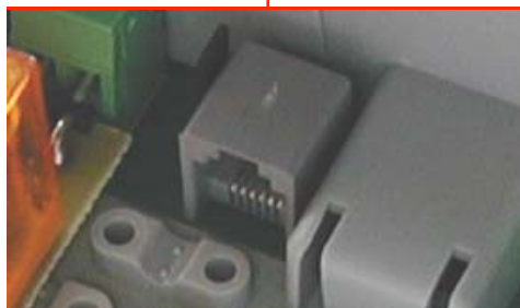
Plug-in 141 2-wire BUS Communication: Supplied cable plugged into control and opposite end is terminated in communication board of HK control
