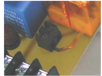
Alarm Connection: Dry contact connection for alarm notification.
